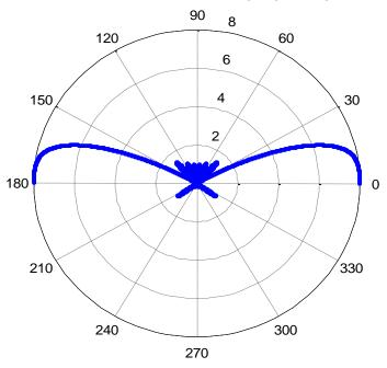
Fig:b:polar plot of N=8 at 0=0deg
