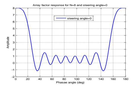
Fig a: phase scanning of N=8,at 0=0deg(plot)
